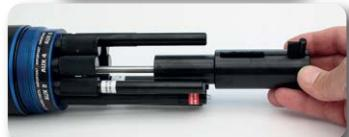
The wiper brushes will keep all sensors clean during the deployment, this is particularly important for the optical sensors that use lenses for measurement.
