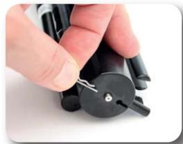
Top: Remove the pin from the top of the cleaning arm
